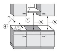
There must be a safety distance of at least 30" (760 mm), ③ between the appliance and any objects above it. The overhead cabinet depth, ④, if unprotected, must not exceed 13" (330 mm). The minimum distance of combustible surfaces located above and to the sides of the cooktop, ⑤, is 18" (457 mm).
