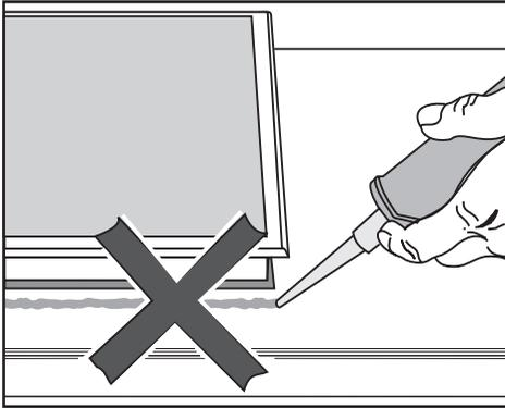
The cooktop must not be permanently sealed into the countertop when installed. The sealing strip under the edge of the cooktop provides a sufficient seal.
