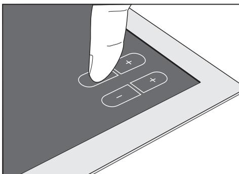
Take care to touch only the desired sensor switch in the middle with your finger vertical, and keep the control panel clean with nothing placed on top of it. Otherwise, the sensor areas may not respond, or unintentional commands may be given, even causing the cooktop to automatically switch off (see the section on "Safety Switch-Off"). NEVER place hot cookware on the sensor switches. The electronic unit underneath might be damaged.
