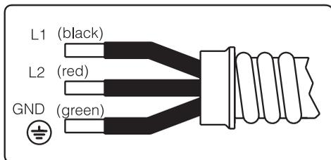
A dedicated line and junction box should be used to connect the cooktop to a 50 A circuit.
