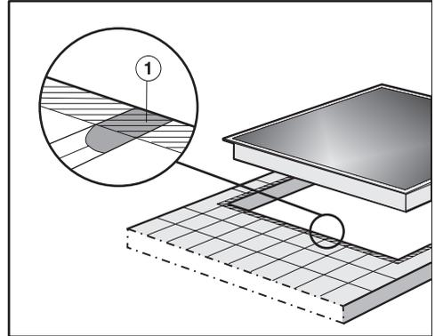
Grout lines ① and the hatched area underneath the cooktop frame must be smooth and even, so that the frame will sit flush with the countertop and the sealing strip underneath the edge of the upper part of the appliance provides a sufficient seal between the cooktop and the countertop.
