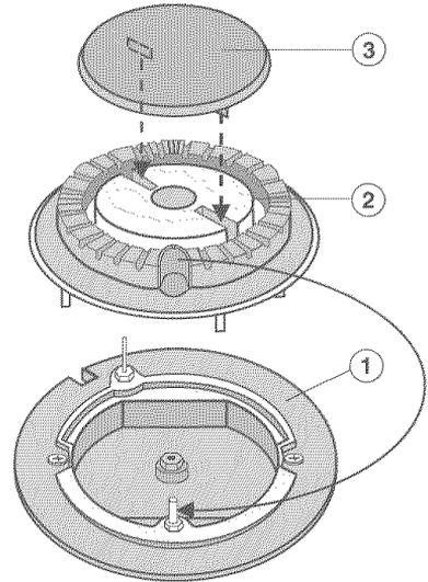
Be careful not to mix up the parts. Make sure that all the locating tabs and notches align exactly.
