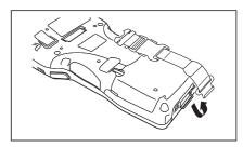
2. Pull on the hand strap in the direction shown in the illustration, and then fasten Hook A onto hook (1) on the back of the Handheld Printer Terminal.
