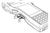
2. Pull out the SD memory card and close the cover of the SD memory card slot.
