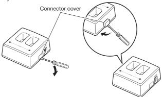
2. Connect the two Dual Battery Chargers as shown below.
