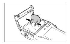
3. Insert the attachment of the 58 mm Paper Width Adjuster into the mounting holes inside the left side of the printer cover to lock in position.
