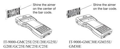
2. The Handheld Printer Terminal reads the code by emitting laser and red lights. Indicator 2 (read operation indicator lamp) lights in green when the reading is successful.
