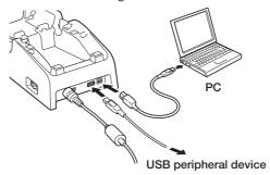
Turn on the power switch on the right side of the USB Cradle. The power LED on the top of the USB Cradle lights red.
