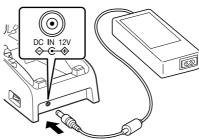
2. After connecting the power cable to the AC adaptor, plug the other end of it into an electrical outlet.
