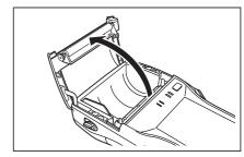
4. Peel off the seal from the roll paper and install as shown in the illustration.
