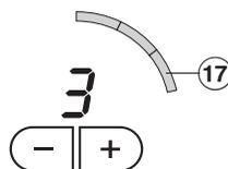
You can increase or decrease the continued cooking setting at any time during the auto heat time with the + or - touch controls. The heat-up time will adjust accordingly.
