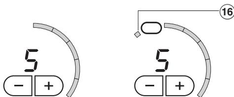
The extended burner is controlled by the touch controls of the rear middle right burner.
