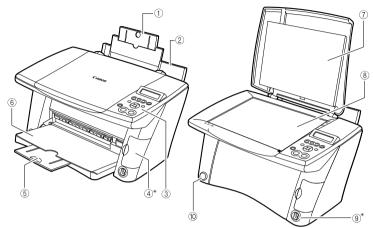
① **Tray extension** Supports paper loaded on the multi-purpose tray. Pull it out before loading paper.
