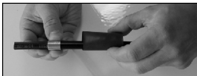
Figure 51: Placing the Heat Shrink Tubing and Ferrule
