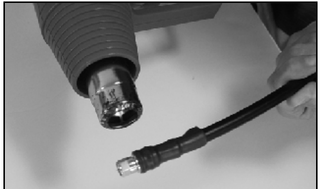
Figure 62: Applying the Heat Shrink Tubing
