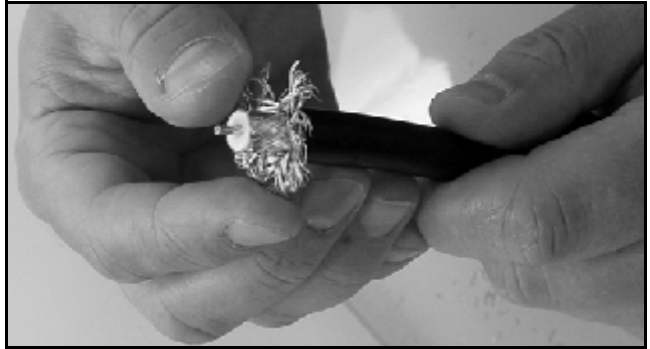
Figure 57: Flaring the Braid
