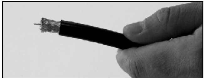
Figure 55: Cable Stripped, Exposing Dielectric
