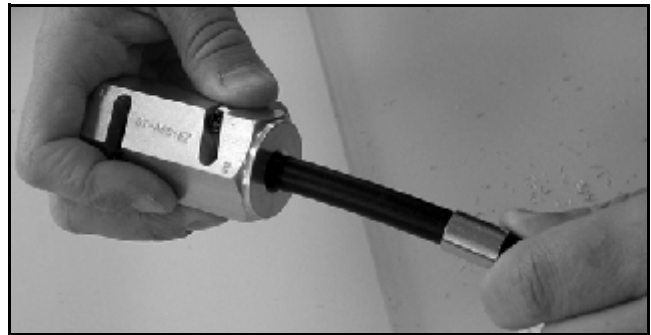
Figure 54: Stripping the Cable Jacket
