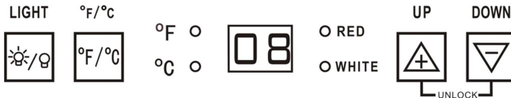
You can select temperature display setting from Fahrenheit to Celsius degree by pushing the button. (Fahrenheit or Celsius indicator will appear in green color) The degrees will appear in blue color in the temperature display window.
