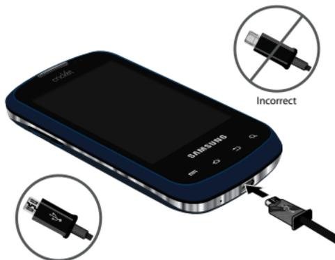
3. Insert the USB cable into the port (2).
