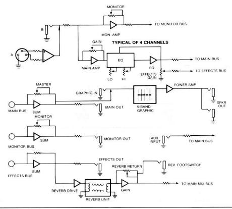
THIS BLOCK DIAGRAM SHOWS SIGNAL FLOW WITHIN THE UNIT. IN ORDER TO THOROUGHLY UNDERSTAND THE UNIT'S FUNCTIONS, PLEASE STUDY THE BLOCK DIAGRAM CAREFULLY.
