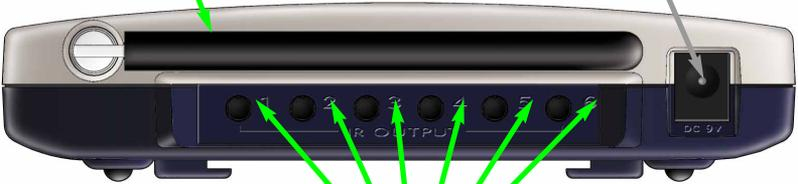
Six Rear Flasher Line Output Jacks connect flashers for control of A/V components out of sight of the MRF-200's Front Blaster.
