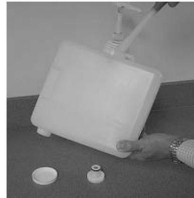
FIGURE 2. Remove Cap and Nozzle Adapter and Clean with Hot Water and Mild Dish Detergent using the Brush.
