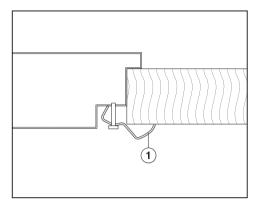
■ Secure the cooktop in position with the supplied fixing brackets, ①.
