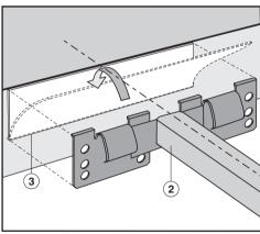
■ Position and attach the spring clips
