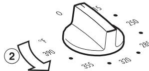
Do not turn the fryer on without pressing the control knob down, and do not turn the knob past "400" to reach "0".
