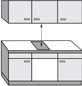
The minimum safety distance given by the hood manufacturer must be maintained between the fryer and the hood above it. See the installation instructions of the hood for these safety measurements.
