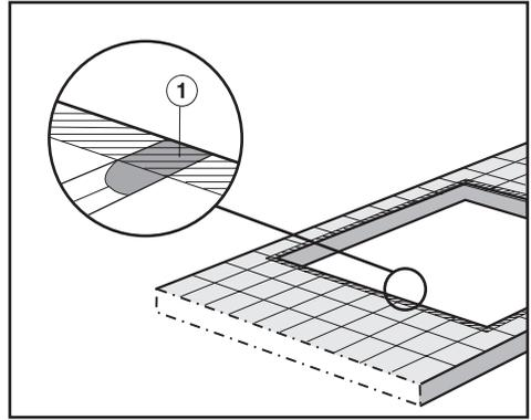
The grouting ① and shaded area under the appliance frame must be flat and even so that the frame will lie evenly and the sealing strip under the edge of the upper part of the appliance can provide an adequate seal against the countertop.
