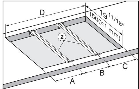
For the installation of **three appliances** the width of the countertop cut-out D is the sum of A and B and C.
