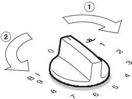
The knob must only be turned clockwise to turn the burner on and counterclockwise to turn the burner off.
