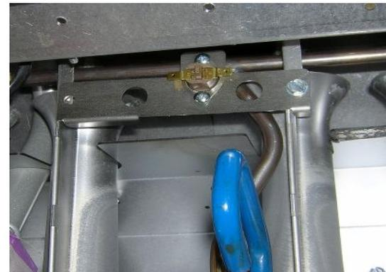
You have now successfully installed the Pitco Self-Cleaning Burner system. Apply the schematic label provided with the kit over the one on the inside of the appliance door. **Before proceeding it is highly recommended that you now thoroughly check the appliance to insure that the procedure was properly followed. Check that all gas joints are tight, all electrical connections are correct, and that the appliance is completely and properly reassembled.**
