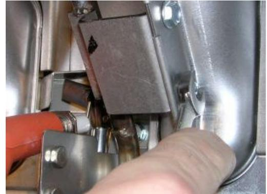
The SCBS Arm should now be mounted properly and securely. Inspect your work to insure that the burners are installed correctly. Improperly mounted or poorly aligned burners may result in an unsafe condition or poor appliance performance. They should be mounted properly on the orifice fittings, facing straight into the burner tubes and secured tightly to the appliance.
