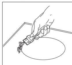
**Burnt sugar** and melted plastic must be removed immediately, when they are still hot, with a glass scraper. Then clean the hob again as described under Item 2.
