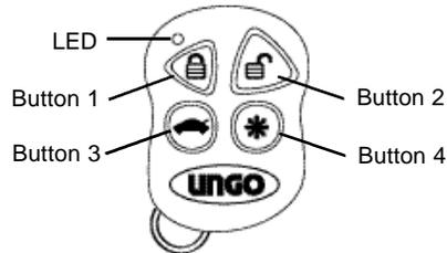
The Ungo MS2004 comes with 2 multi-function Remote Transmitters used to control nearly all of the system's features.
