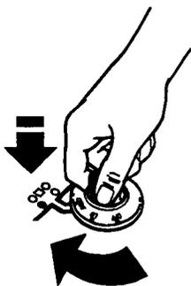
2. After the burner lights, turn the control knob to the desired setting.
