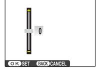
To determine the amount required, adjust peripheral illumination correction while taking photos of blue sky or a sheet of gray paper.
