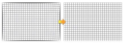
To determine the amount required, adjust distortion correction while taking photos of graph paper or other objects featuring repeating vertical and horizontal lines, such as the windows in a high-rise.
