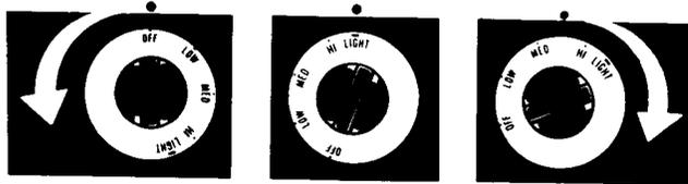
When the burner is lit, turn the control knob to the right to the desired flame setting, see guide below. The control knobs do not have fixed positions between "HI" and "LO". They can be turned to any of the settings indicated, or to any position in between. The ignitor will turn off and the clicking will stop when the control knob is turned from the "LIGHT" position to another setting.
