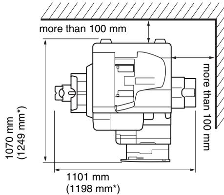
\* When the left cover of the main unit is opened and the auxiliary tray of the Additional Finisher Tray-C1 is extended.
