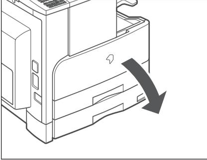
**2** While pushing down the release tab, turn the toner cartridge in the direction of the arrow in the illustration below.
