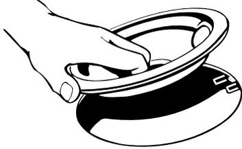
3. Hold the coil element as level as possible with the terminal just started into the receptacle. Push the coil element terminal into the receptacle.
