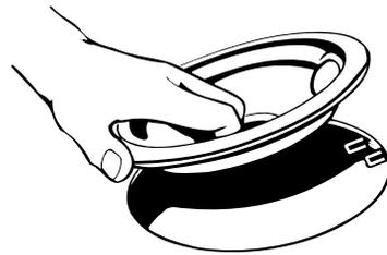
2. Push in the edge of the coil element, opposite the receptacle. Then lift it just enough to clear the reflector bowl.
