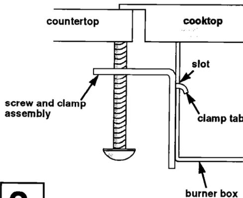
**3.** Insert one clamp tab through each slot located on sides of the burner box.
