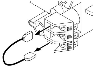
**Figure 36 - Connecting Wall Switch to Control Cover**
