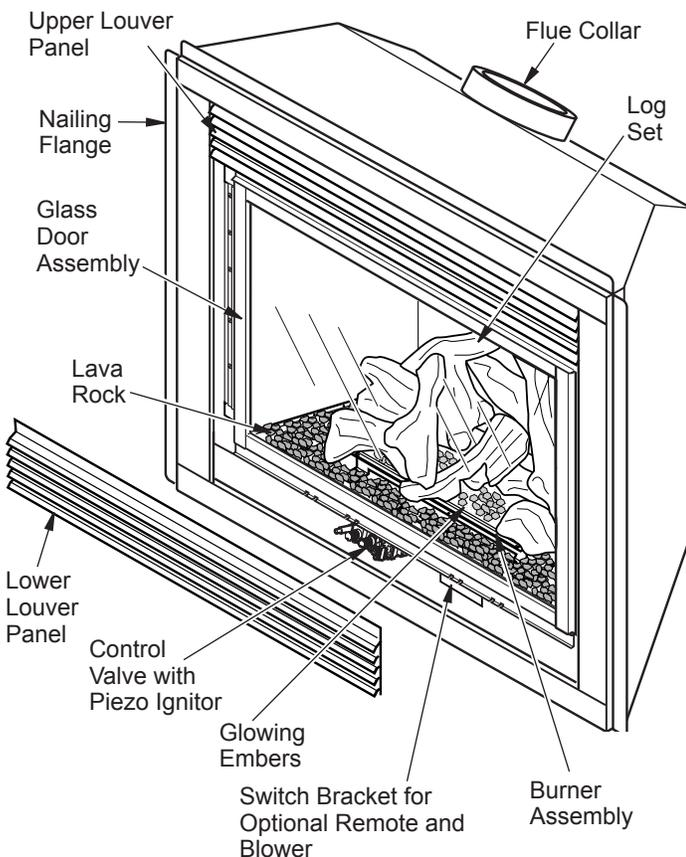
Figure 1 - Direct-Vent Fireplace with Millivolt Ignition
