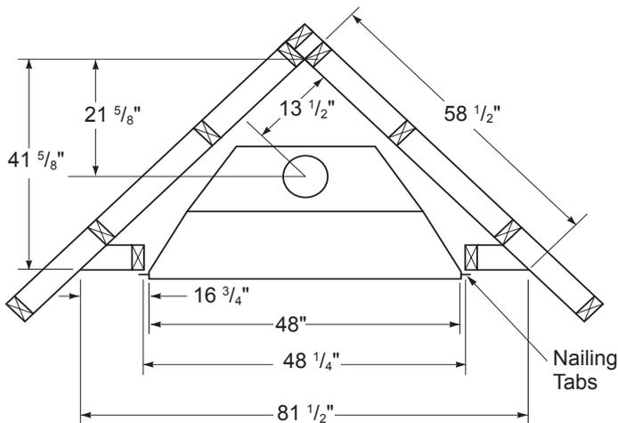
**Figure 5 - Framing Clearances for Corner Installation**
