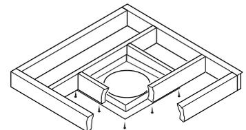
**Figure 20 - Installing Firestop**
