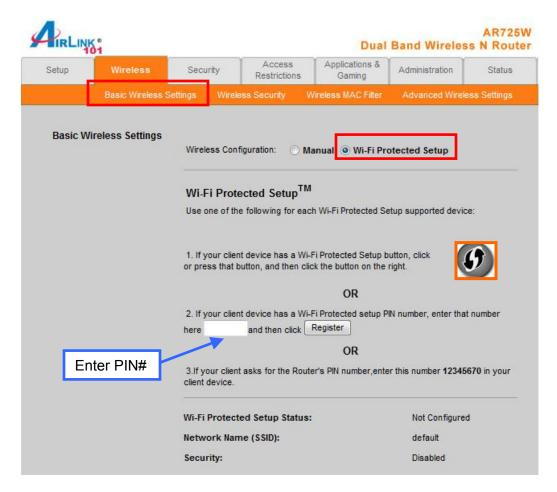
WiFi Protected Setup supports two types of connection: Push Button Configuration (PBC) or Personal Identification Number (PIN).
