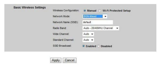
**Network Mode**: If you have 802.11b/g/n 2.4GHz devices on the wireless network, select **BGN-Mixed**. If you have 802.11a/n 5GHz devices on the wireless network, select **AN-Mixed**.
