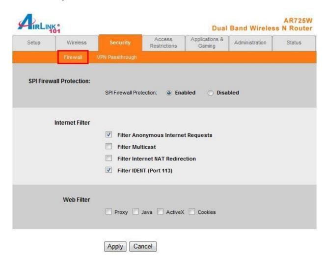
SPI Firewall Protection: Select to enable or disable Stateful Packet Inspection.
