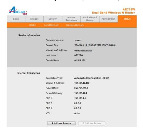
If you see all 0's, click on the **IP Address Renew** button (for Cable Modem users) or the **Connect** button (for DSL users).
