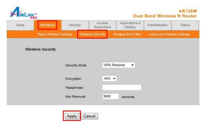
**Encryption**: Select either **TKIP** or **AES** or **AES** as the encryption method.
