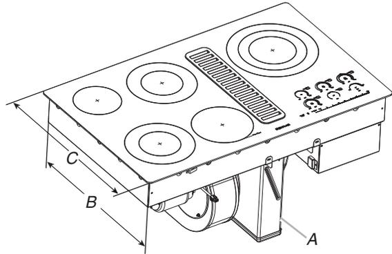
A. Model/serial rating plate location
