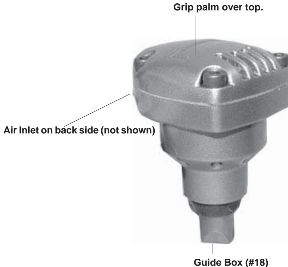
4. Holding an 8D, 9/32" nail by the stem (not the tip), insert the head of the nail into the **Guide Box (#18)**, and grip your palm over the top of the Nailer. See **FIGURE 1**.
