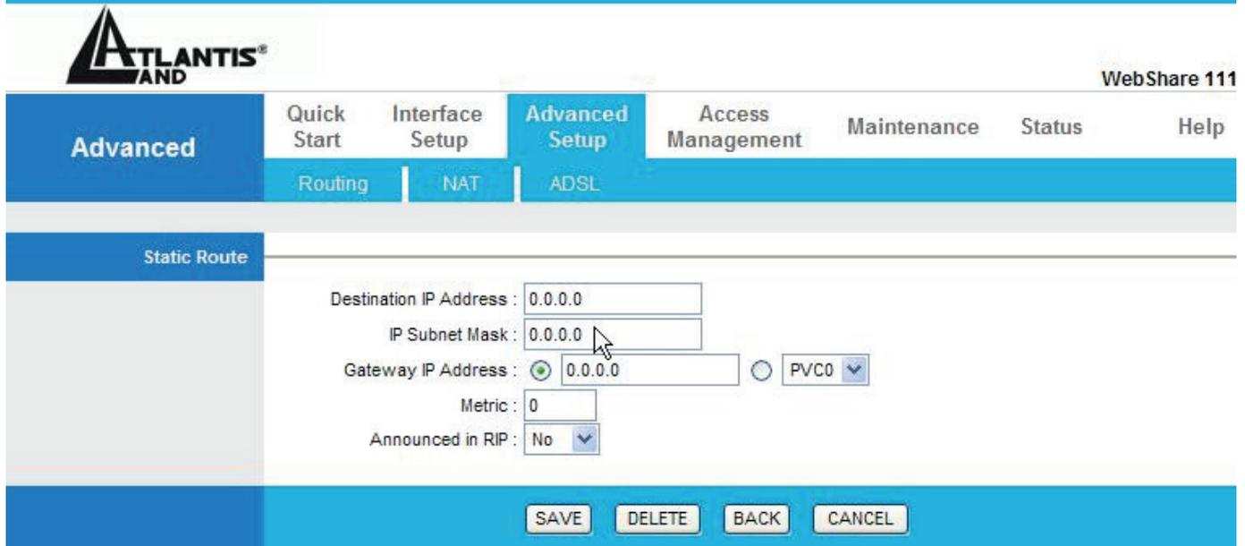
The screenshot shows the Atlantis WebShare 111 interface. The top navigation bar includes 'Quick Start', 'Interface Setup', 'Advanced Setup', 'Access Management', 'Maintenance', 'Status', and 'Help'. Under 'Advanced Setup', there are sub-tabs for 'Routing', 'NAT', and 'ADSL'. The 'Static Route' configuration page is displayed, featuring the following fields:
