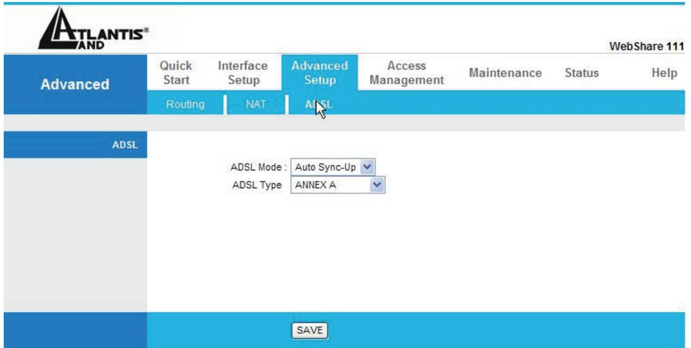
The screenshot shows the Atlantis AND WebShare 111 configuration interface. The top navigation bar includes 'Advanced', 'Quick Start', 'Interface Setup', 'Advanced Setup', 'Access Management', 'Maintenance', 'Status', and 'Help'. Under 'Advanced Setup', there are sub-tabs for 'Routing', 'NAT', and 'ADSL'. The 'ADSL' sub-tab is active, showing two dropdown menus: 'ADSL Mode' set to 'Auto Sync-Up' and 'ADSL Type' set to 'ANNEX A'. A 'SAVE' button is located at the bottom of the configuration area.
