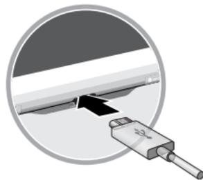
1. Insert the USB cable into the port.
