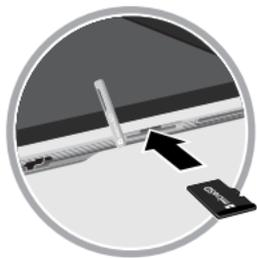
1. Open the microSD card slot cover and turn to expose the slot.
