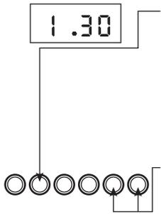
**Step 4** Press & hold in the Cook Period button, the display will read 0.00 and the 'cookpot' symbol will light up. With the Cook Period button still held in set the required Cook Period using the "+" and "-" buttons. Example: 1hr 30 minutes (as shown).
