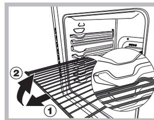
**WARNING !** The oven is provided with a stop system to extract the racks and prevent them from coming out of the oven (1).
