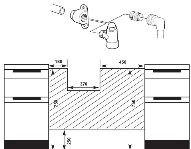
Connection to the cooker should be made with an approved appliance flexible connection in accordance with current National legislation. A length of 0.9 to 1.25m is recommended. The length of hose chosen should be such that when the cooker is in situ, the hose does not touch the floor.
