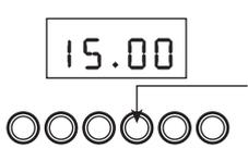
**Step 2** Press the Manual button to return the oven to "Manual" operation. The 'Auto' symbol will go out.
