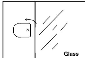
3. The inside of the outer door glass can now be cleaned while still fitted to the cooker.
