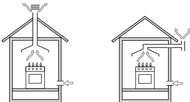
In a chimney stack or branched flue.
