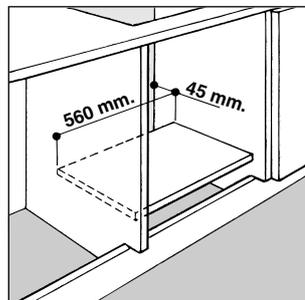
When installing the hob above a built-in oven without forced ventilation, ensure that there are air inlets and outlets for ventilating the interior of the cabinet adequately.
