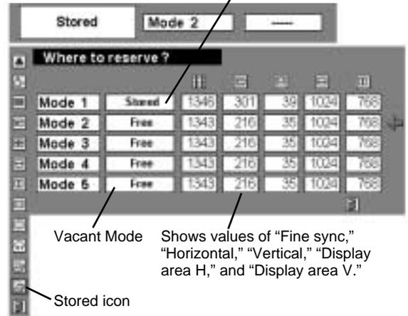
Vacant Mode Shows values of "Fine sync," "Horizontal," "Vertical," "Display area H," and "Display area V."
