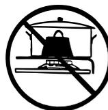
Do not use large pots or heavy weights which can bend the pan support or deflect the flame onto the hotplate.
