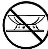
Do not remove the pan support and enclose the burner with a work stand as this will concentrate and deflect the heat onto the hotplate.
