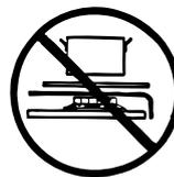
Do not place anything, e.g. diffuser, asbestos mat, between pan and pan support as serious damage to the appliance may result.
