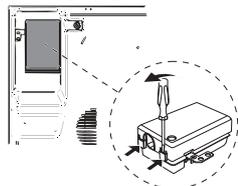
On the lower part of the appliance there is a connection box for the different types of electricity supply (the picture is only an indication and is not an exact representation of the purchased model).
