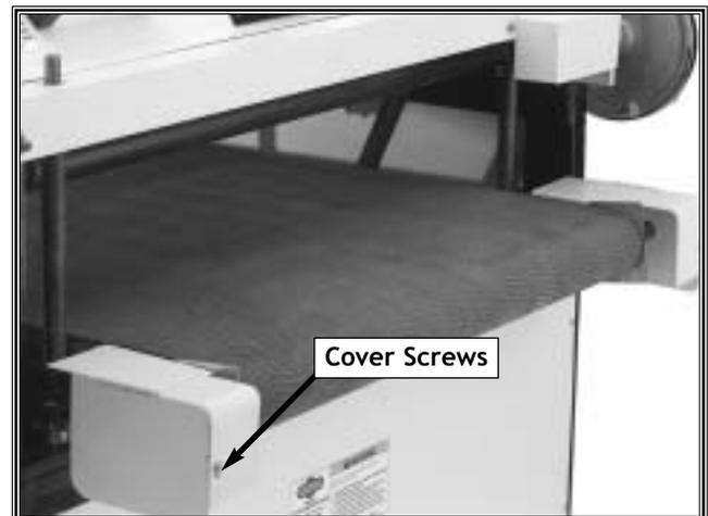
**Figure 40.** Infeed-conveyor safety covers.
