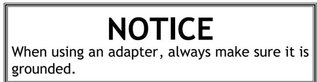
Remember, an adapter with a grounding wire does not guarantee the machine will be grounded. A ground source must always be verified in the electrical circuit within the wall or conduit.
