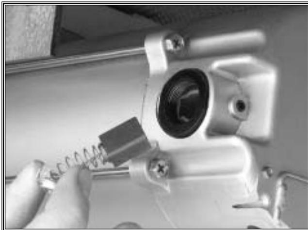
**Figure 55.** Carbon brush and spring.
