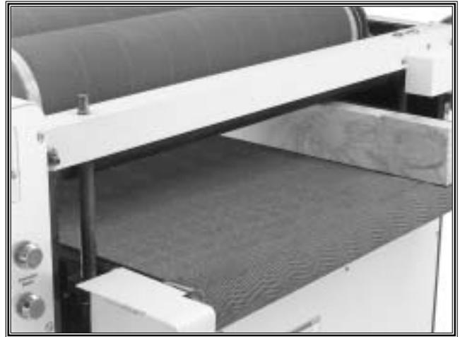
**Figure 28.** The 30" gauge block positioning.
