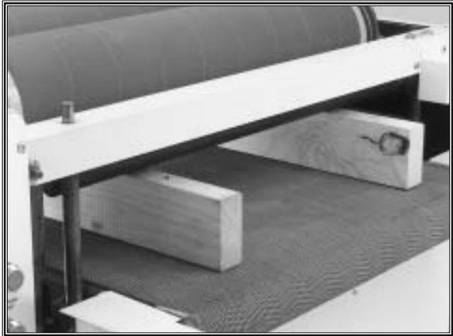
**Figure 35.** Two gauge blocks in position.
