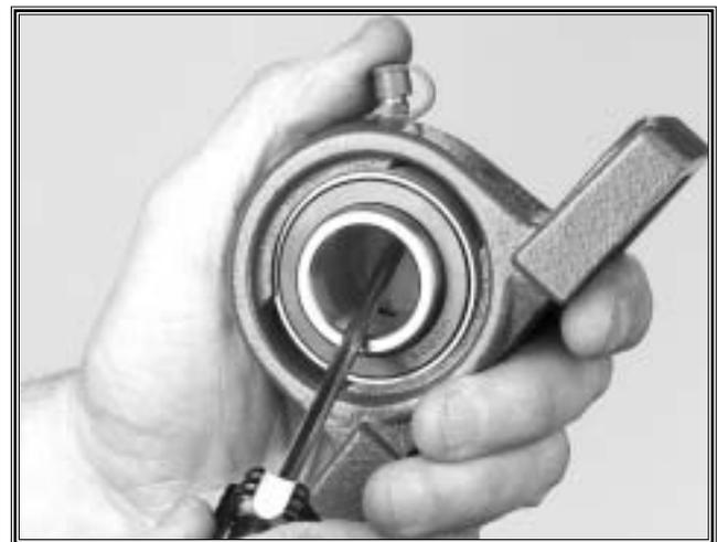
Figure 58. Bearing positioning for removal.
