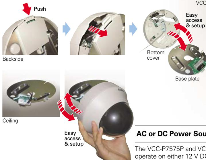
After fastening the base plate at the point of surveillance, installation is completed by simply snapping on the bottom cover and the camera unit.
