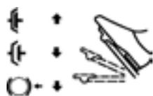
1. Pedal released – service brake not activated.
