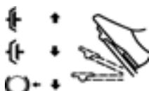
1. Pedal released – forward drive engaged. The machine will move if a gear is engaged. Service brake not activated.
