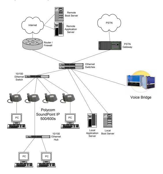
The phones connect physically to a standard office twisted-pair (IEEE 802.3) 10/100 megabytes per second Ethernet LAN and send and receive all data using the same packet-based technology. Since the phone is a data terminal, digitized audio being just
