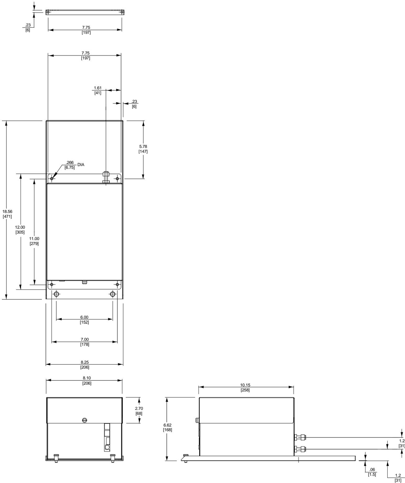
**Figure 2-2. Trace Oxygen Analyzer Outline and Mounting Dimensions**
