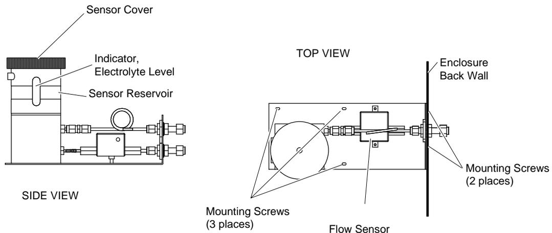
**Figure 4-1. Trace Oxygen Analyzer Sensor Assembly**
