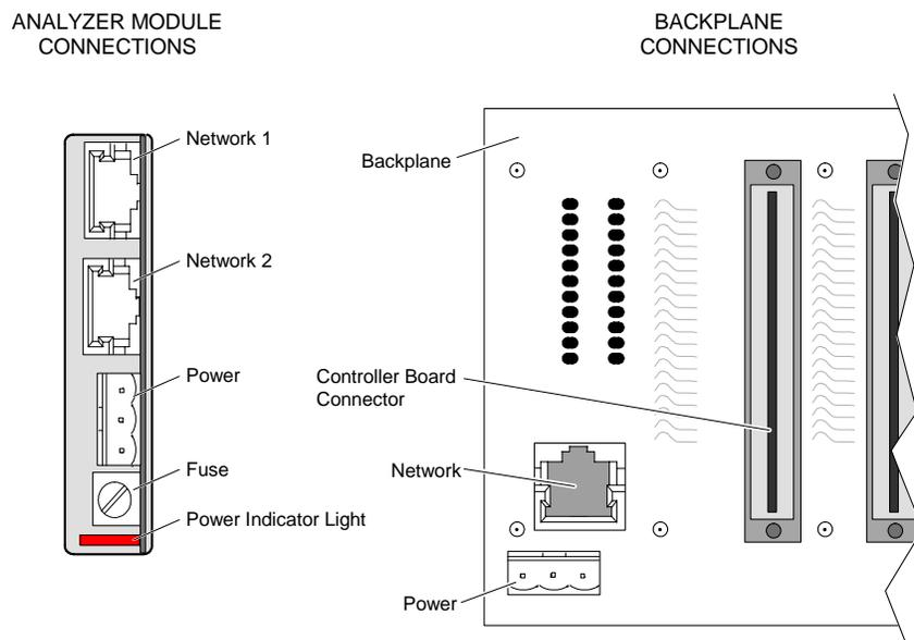
**Figure 2-1. Analyzer Module Interconnection with Instrument Platform**
