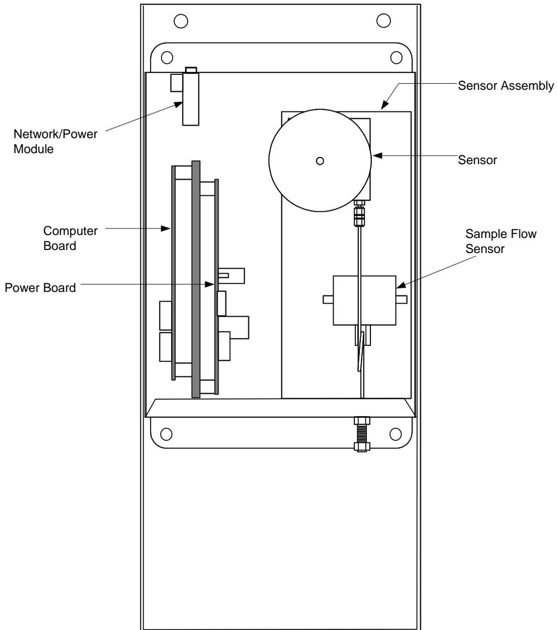
**Figure 1-2. Trace Oxygen Analyzer Module – Top View**
