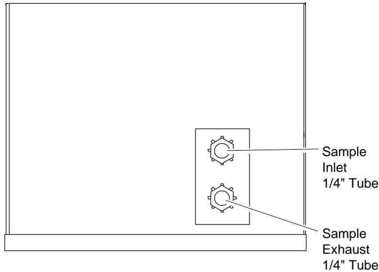
Figure 2-3. Trace Oxygen Analyzer Back Panel Connections
