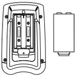
The Bonus Receiver use 2 x AA, IEC LR6, 1.5V batteries. When the batteries need to be replaced, the low battery symbol will appear on the LCD. To install and replace the batteries, please follow the steps below:
