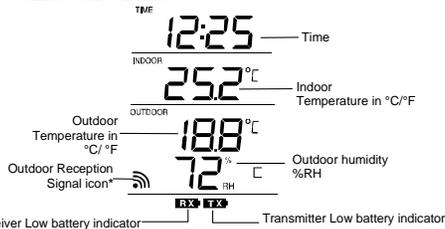
\* When the signal is successfully received by the Bonus Receiver, the outdoor reception icon will be switched on. (If not successful, the icon will not be shown on the LCD) So the user can easily see whether the last reception was successful (icon on) or not (icon off). On the other hand, the short blinking of the icon shows that a reception - is being done currently.
