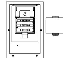
The Weather Center works with 3 x AA, IEC LR6, 1.5V batteries. When the batteries need to be replaced, the low battery symbol will appear on the LCD.
