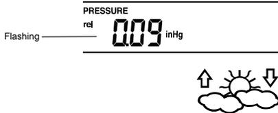
You may select a definite switching sensitivity value, .06, .09, or .12 inHg for the change in the display of weather icons. This represents the "sensitivity" of the weather forecast (the smaller the value selected, the more sensitive the weather forecast). The default value is 0.09 inHg.
