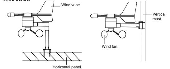
Firstly, check that the wind-fan and the wind-vane can rotate freely before fixing the unit. For correct and accurate readings it is important to mount the sensor so that the front (marked E) is pointing in East-West direction. The wind sensor should now be
