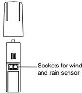
2. First insert the batteries into the Thermo-hygro sensor (see **"How to install and replace the batteries into the Thermo-hygro sensor"** below).
