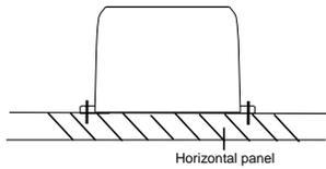
For best results, the rain sensor should be securely mounted onto a horizontal surface about 2-3ft (60-90cm) above the ground and in an open area away from trees or other coverings where rainfall may be reduced causing inaccurate readings.
