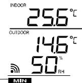
2. Press the **min/max/+** key once more to view the maximum indoor temperature, maximum outdoor temperature and maximum outdoor humidity.
