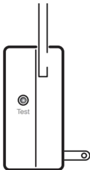
**Step 2** - When the Control Center receives the Signal Repeater's test signal, it will flash the green power indicator. This means a confirmation signal was sent back to the Signal Repeater. Release all buttons.
