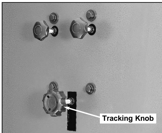
Figure 3. Tracking knob adjustment location.
