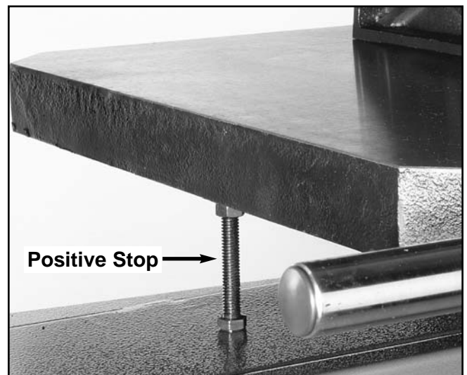
Figure 9. Location of positive stop adjustment.
