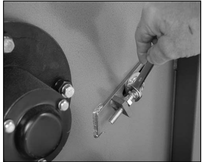
Figure 11. Backing off lock bolt.
