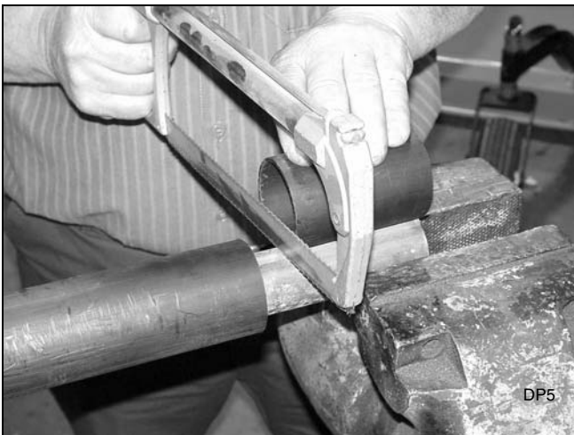
Figure 9. Cut Shaft to Length
