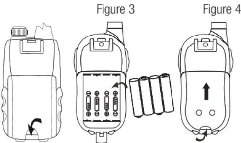
*Caution: Observe the proper battery polarity orientation when installing batteries. Incorrect positioning can damage both the batteries and the unit.*
