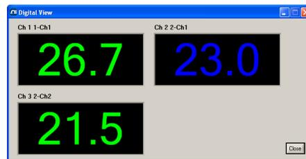
The size of this window will adapt to the number of channels to display. Up to 32 values can be shown. Refresh rate is always 1.0 sec. This window is re-scalable.
