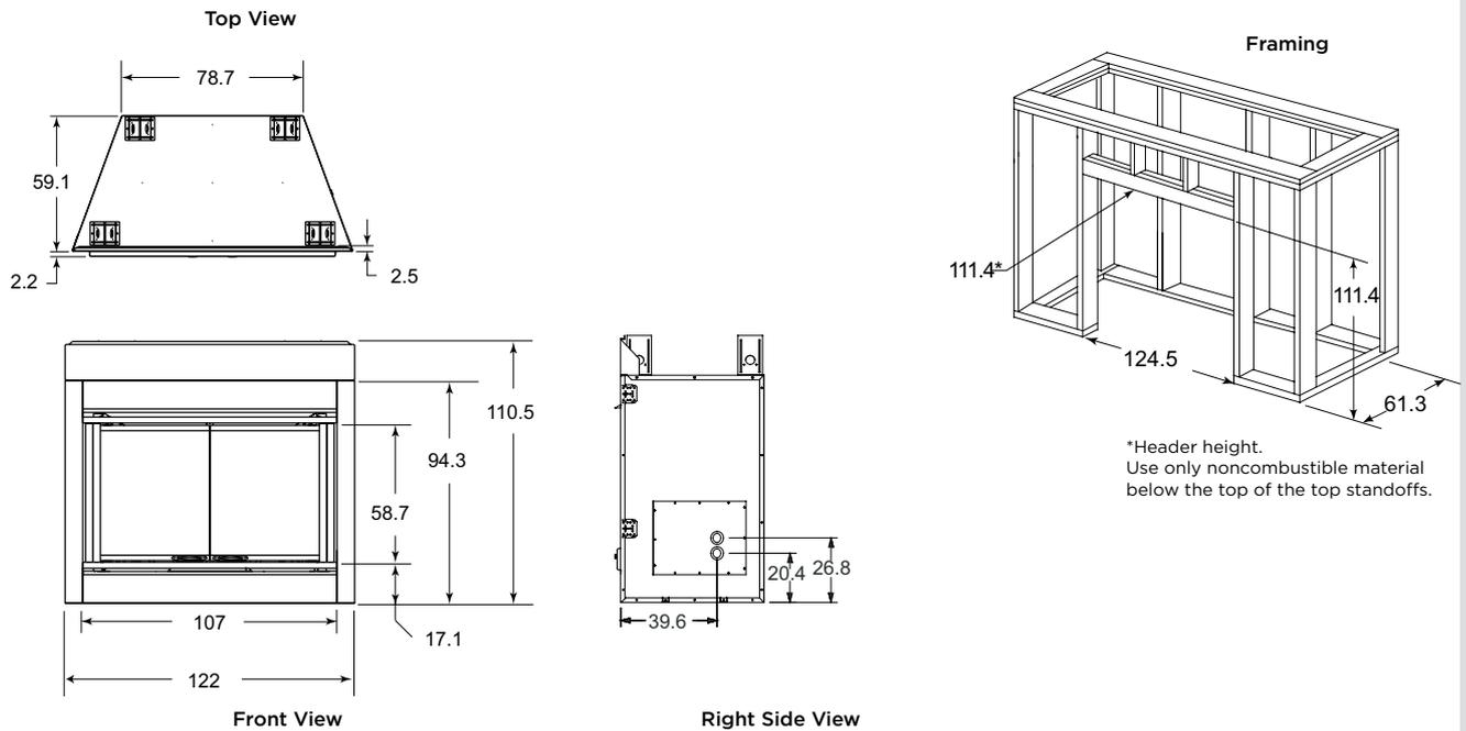
Dimensions above are in centimeters and for reference only. We recommend measuring individual units at installation. Assumes the use of 1.3cm gyprock.
