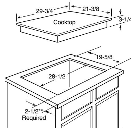
\*Depth of unit at conduit connection location (rear) is 6-1/2" on models PP980/975/950/945 and 4-5/8" on models PHP900/PP972/962/942/932/912, JP655/356/346.
